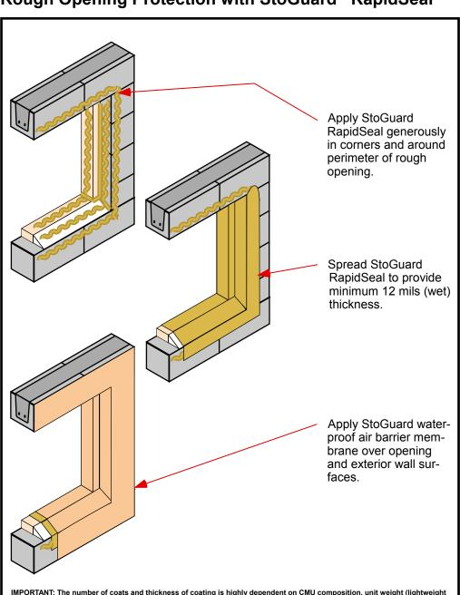
coat the entire wall surface with a Sto base coat, leveling or parging material to fill and level the surface prior to applying the waterproof air barrier membrane and transition materials. When a skim coat of the leveling material is to be applied only one coat of the waterproof air barrier membrane is typically required (refer to Sto Detail 21.00b). Use a site mock-up and site tests as the basis for the work. Property of Sto Corp. All Rights Reserved
